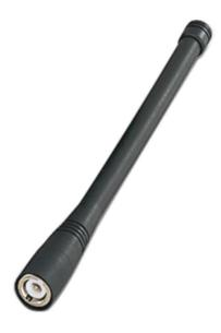
This Icom rubber ducky antenna is compatible with Icom A4, A5, A6, A14, A14S, A22, A23, A24, and A25 radios. This antenna only works for Icom handheld radios and not for panel mount units. Has female BNC connector.
